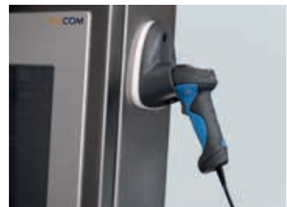
Barcode scanner at monitor enclosure
